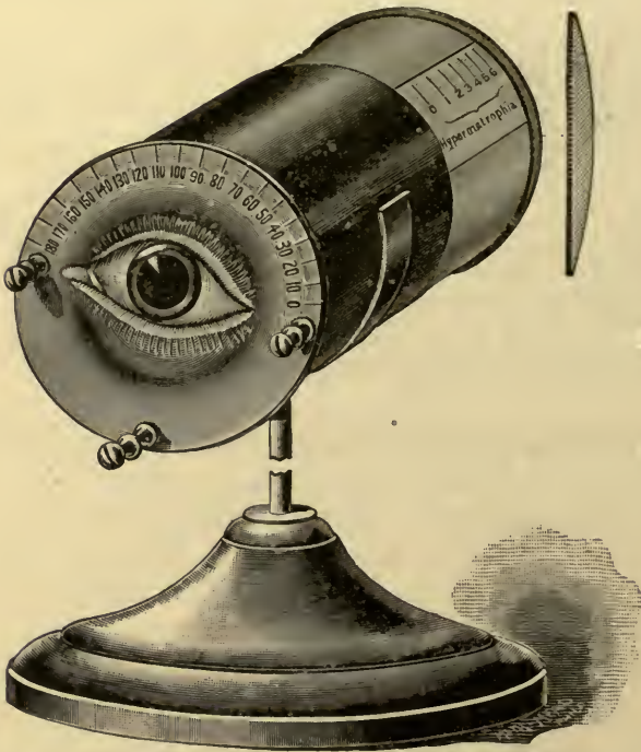
FIG. 143.—The Author's Schematic Eye for Studying Retinoscopy.
